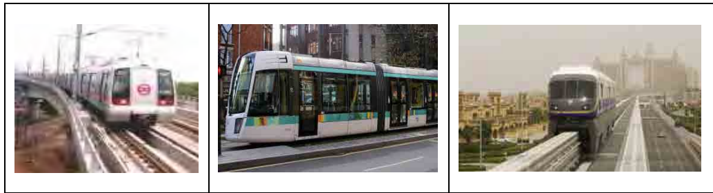
Left to Right: Metro (ex. Delhi), LRT (ex. Paris), Monorail (ex. Dubai)
