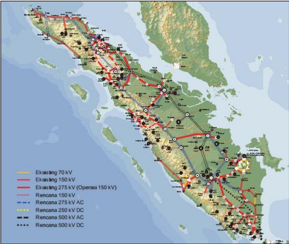
Figure 2-4 Sumatra Grid System Development Plan Source: PLN “2012-2021 Power Development Plan (RUPTL)” Dec 2012
