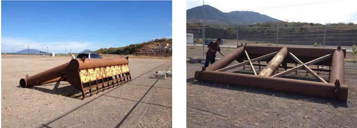
Figure C.12 Photographs of Rake utilized for rake-dredging
