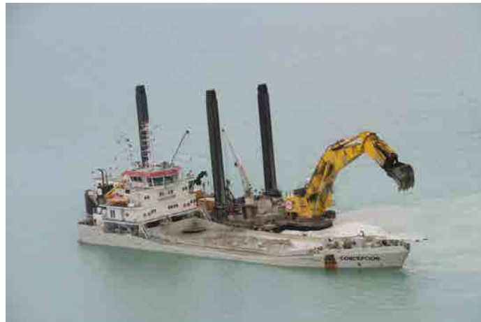
Figure C.46 Photo of Backhoe Dredger (Source: "Mimar Sinan" Jan De Nul Group)
