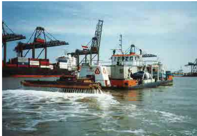
Figure C.18 WID vessel (Source: PIANC Report No. 120-2013 INJECTION DREDGING (J. Smith et al. 2013))
