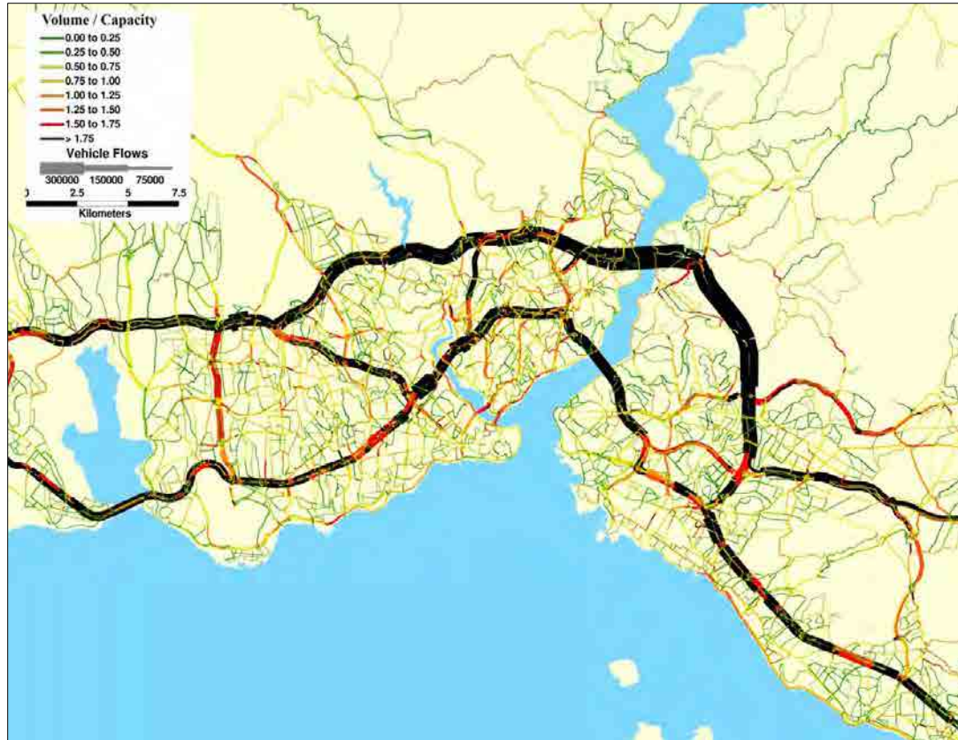
Figure 11 Determination of the congested points as a result of Transportation Master Plan
