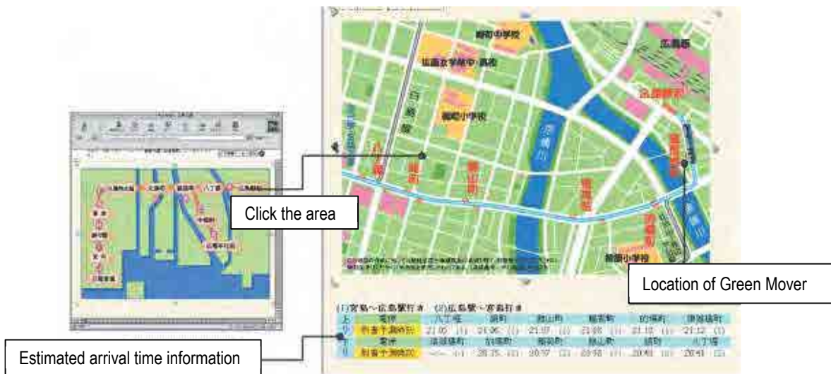
Figure 1.2.3 Bus Location Information System
