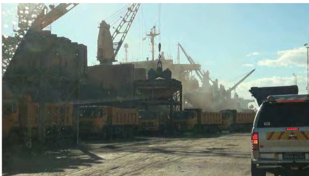
Figure 5.3.10 Bulk Cargo Handling by the Ship's Gear
