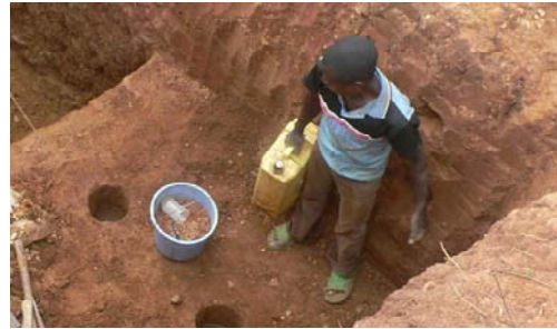
Water splinking and feeding to test hole
