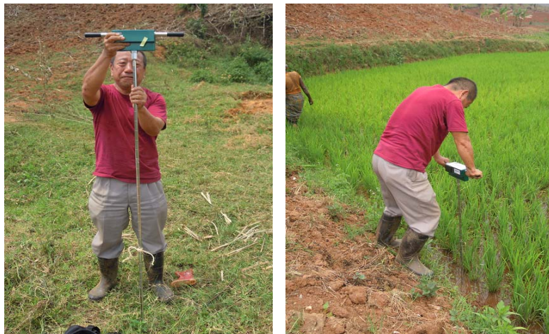
State of cone penetration test
