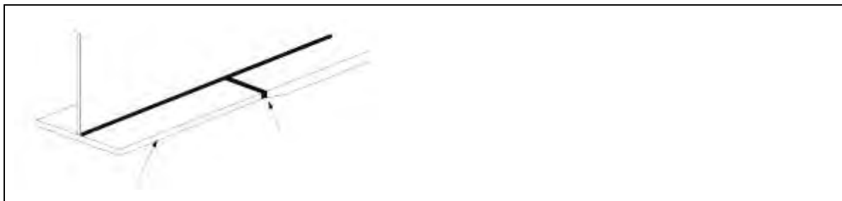
Figure 15.3 Cracks Appearing at Butt Welded Portions on Lower Flanges
