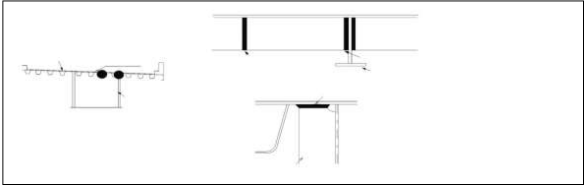
Figure 15.4 Cracks Appearing at Welded Portions with Steel Deck Plates
