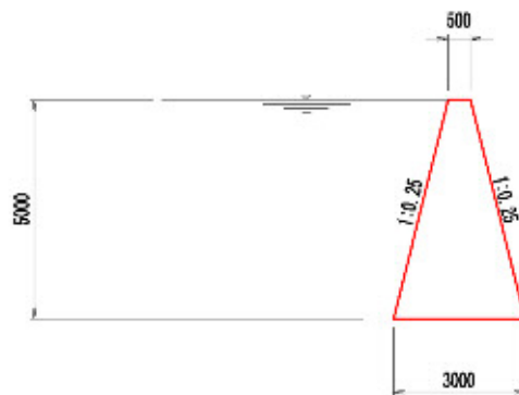
Fig. 2.2.29 Standard Cross-Section of Right-Bank Revetment (Wall Height: 5.0 m)
