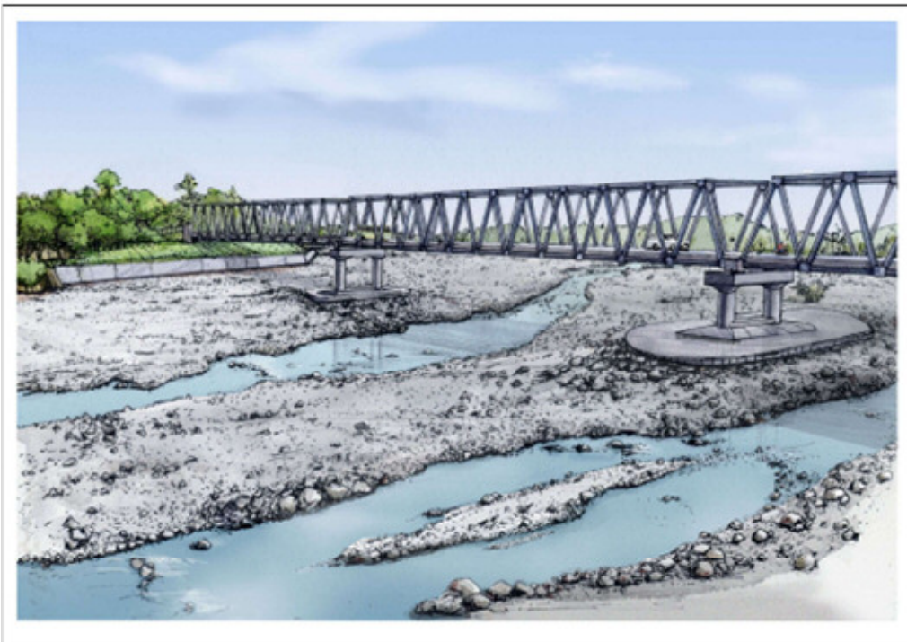
PERSPECTIVE (Protection of Pier and Abutment of the existing Mola Bridge)
