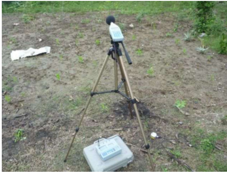
Fig. 1.3.5 Instruments for noise and vibration measurement
