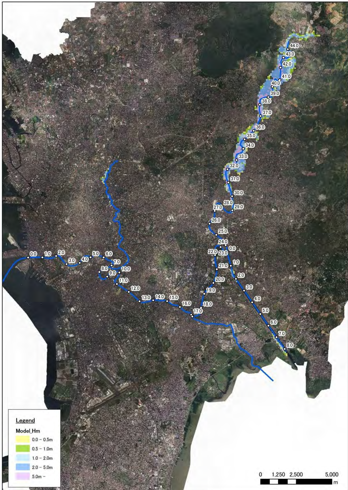
Figure 6.2 Inundation Area by 1/30 Years Flood Without Climate Change Effect
