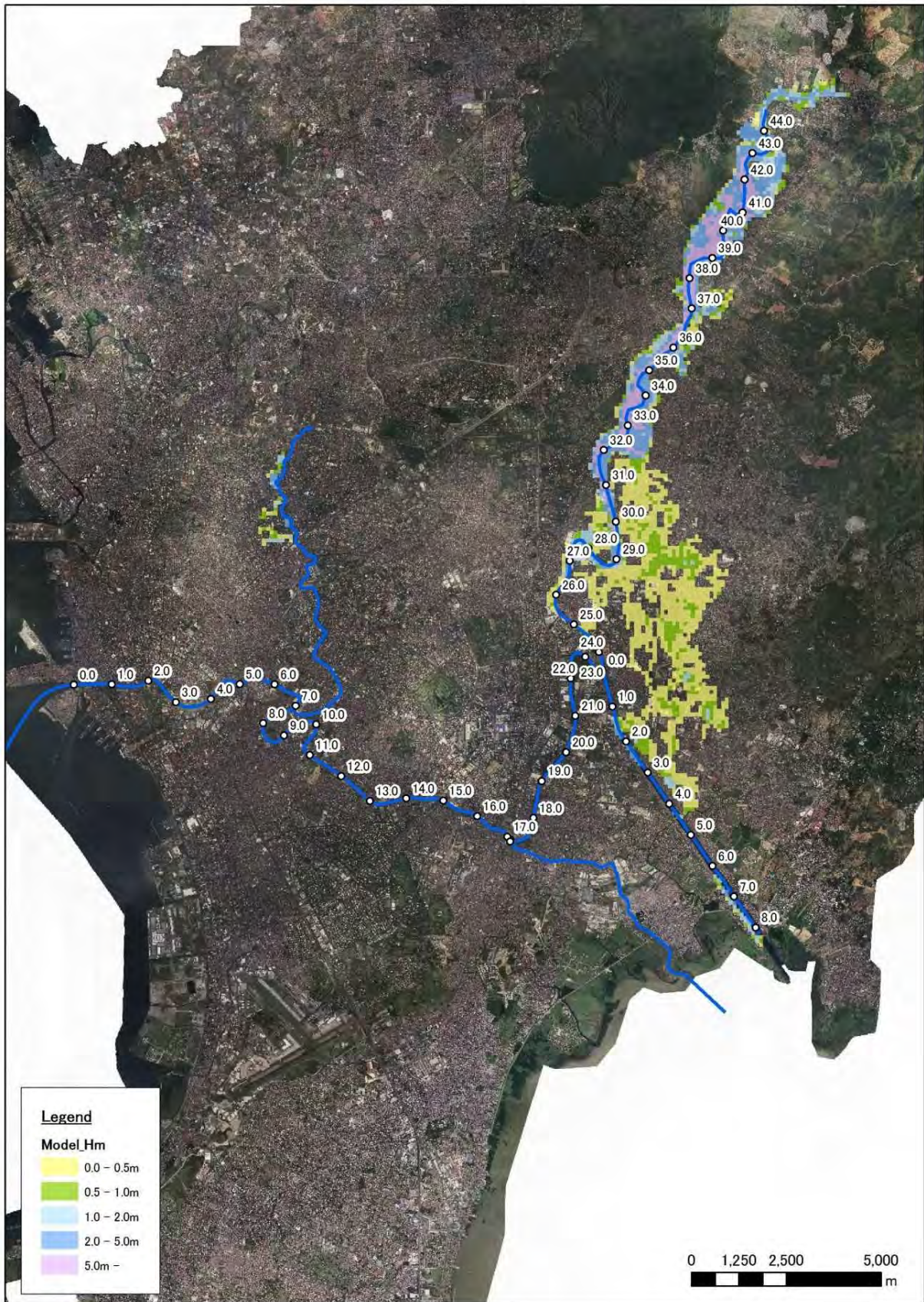
Figure 6.4 Inundation Area by 1/100 Years Flood Without Climate Change Effect
