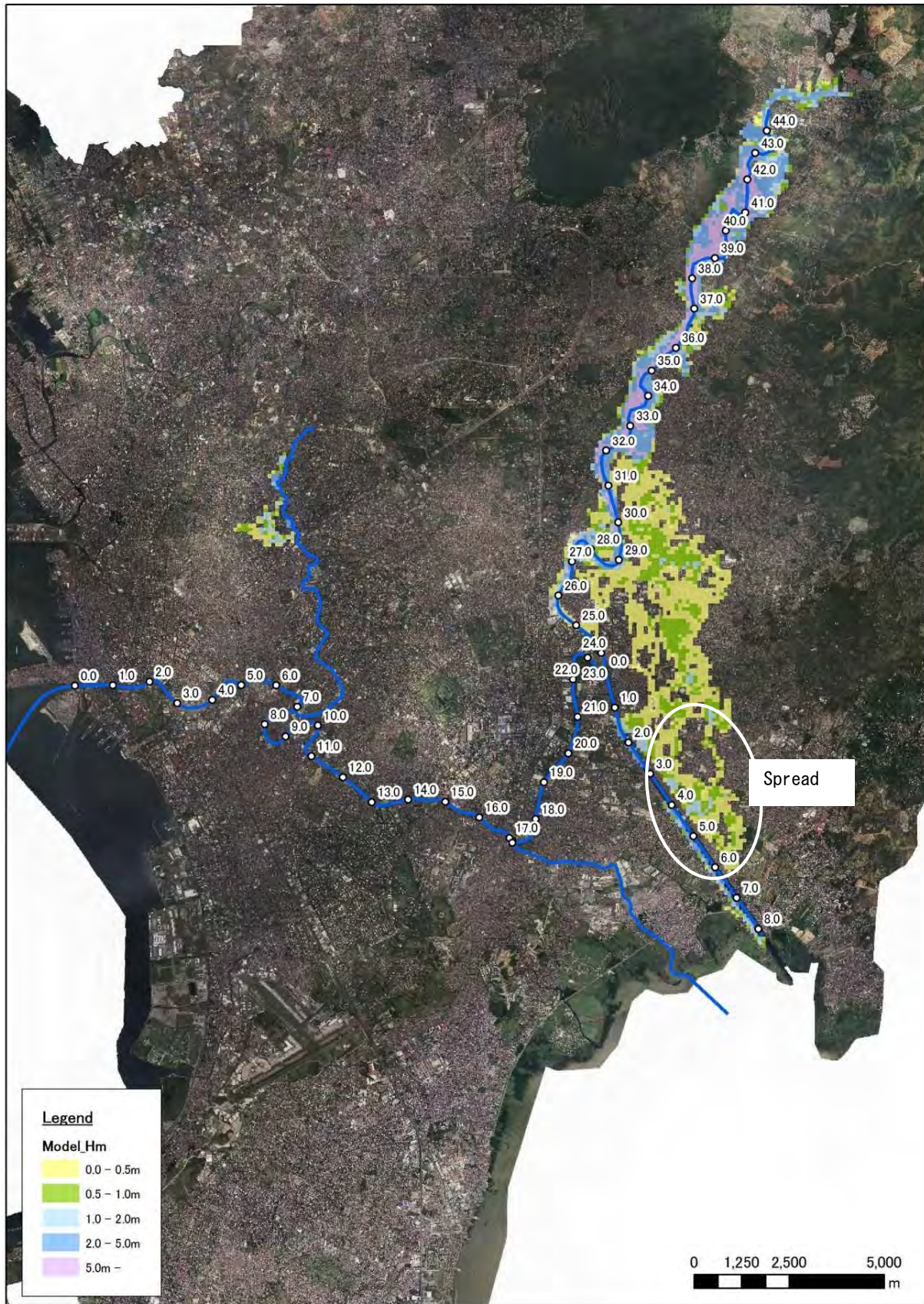
Figure 6.5 Inundation Area by 1/100 Years Flood With Climate Change Effect
