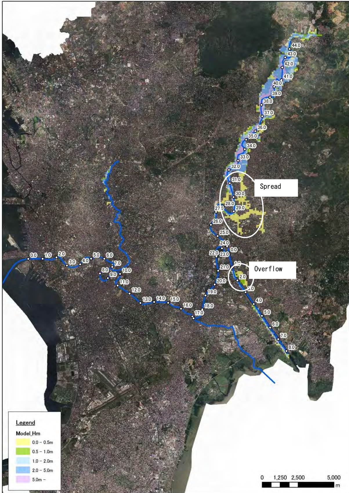
Figure 6.3 Inundation Area by 1/30 Years Flood With Climate Change Effect
