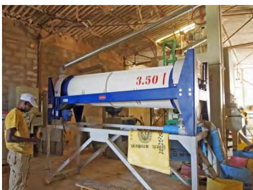
Length grader installed on the existing rice mill. Operated together with the existing rotary sifter. February, 2013 (Ross Bethio area)
