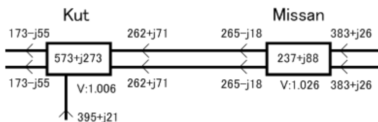
Figure 3.4.6 Precise Power Flow around Missan
