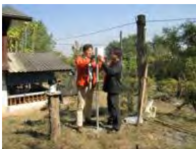
Installing rain gauge
