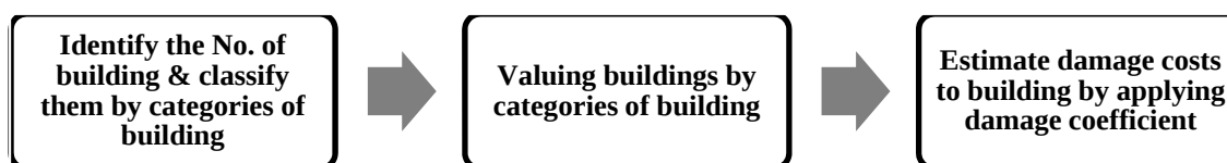
Figure- 4.1.1 Flow Chart for Estimating Direct Damage Costs to Buildings
