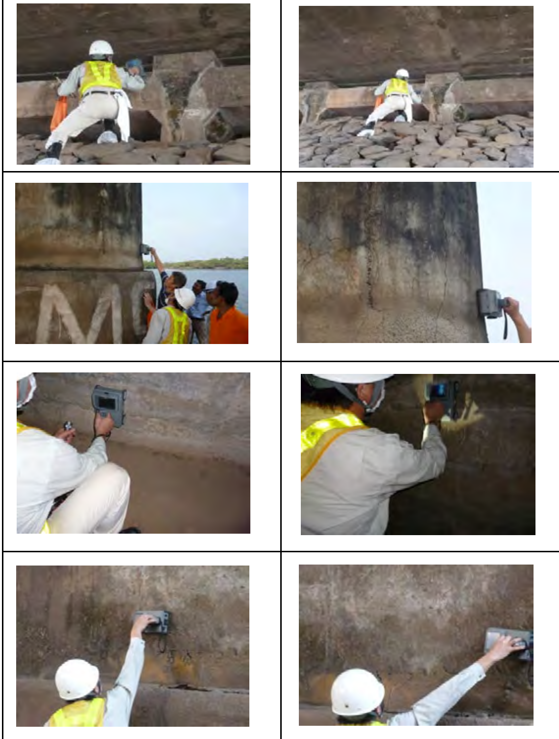
Photos (Concrete cover survey: RC radar)
