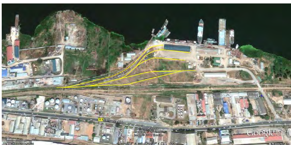
Figure 6.8: Existing Track Layout within Mwanza Port
