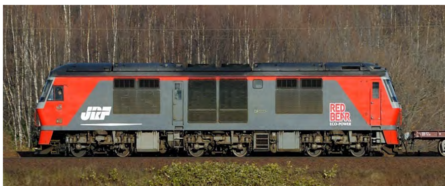
Photo 6.3: Profile View of Toshiba DF 200 AC Locomotive Showing B-B-B (6 Axle) Wheel Configuration
