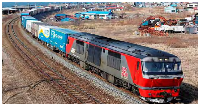
Photo 6.4: Toshiba DF 200 AC at Head of Freight Train
