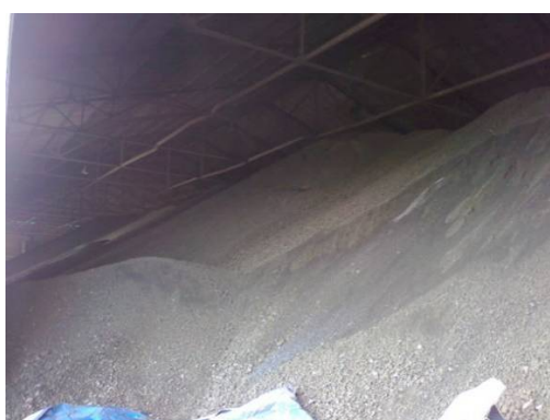
Photo 3.10: Clinker in the Warehouse
