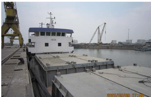
Photo 3.47: Container Fittings on the Hatch Cover of M/S Teza
