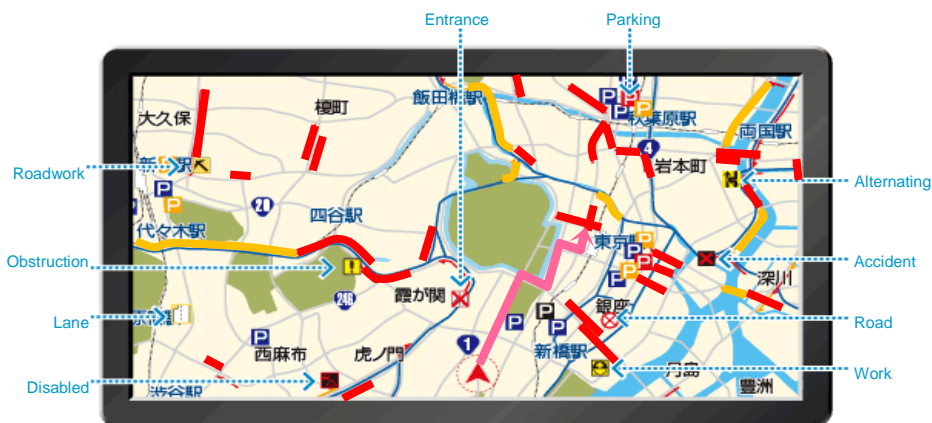
Figure 4-17 Example: Image of Traffic Condition Shown on Car Navigation through VICS
