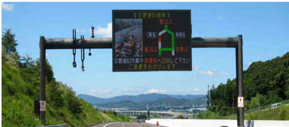
Figure 4-4 Example: Image of Graphic Variable Message Sign Board (Showing road disaster and road closure ahead/ and providing alternative route guidance)
