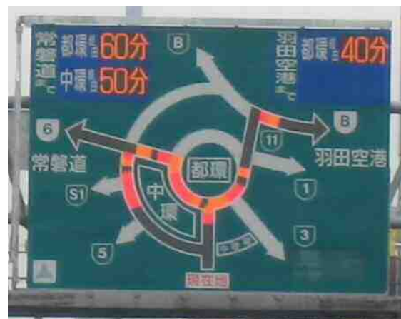
Figure 4-6 Example: Image of Variable Message Signboard (Showing congested section and level of congestion on road network)
