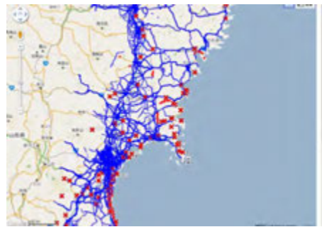
Figure 111 Probe System (Identified damaged road section after massive earthquake in Japan)
