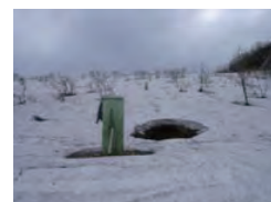
Cave and piezometer
