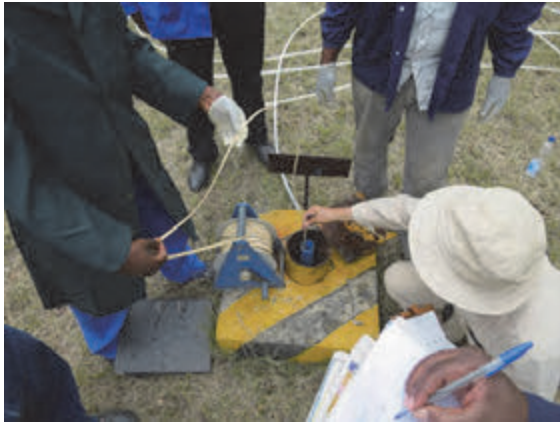
Photo 4.39 Measurement of Water at Monitoring Hole (there are more than ten holes.)
