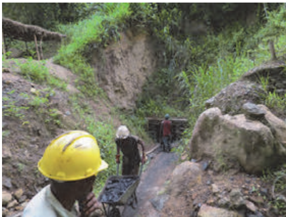
Photo 4.27 Carrying Workers at the Mouth of Drift in Jalawe Coal Mine (small-scale)
