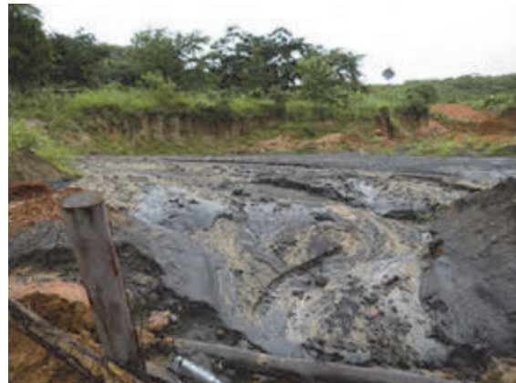
Photo 4.10 Drainage Water and Slag Sump from Washing Plant
