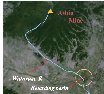
Cu and Fe were deposited in downstream through acidic mine water
