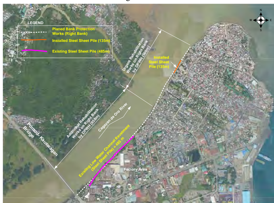
Figure 1.3.3 Location of Urgent Rehabilitation Works and Existing Sheet Piles at Right Bank of the River Mouth
