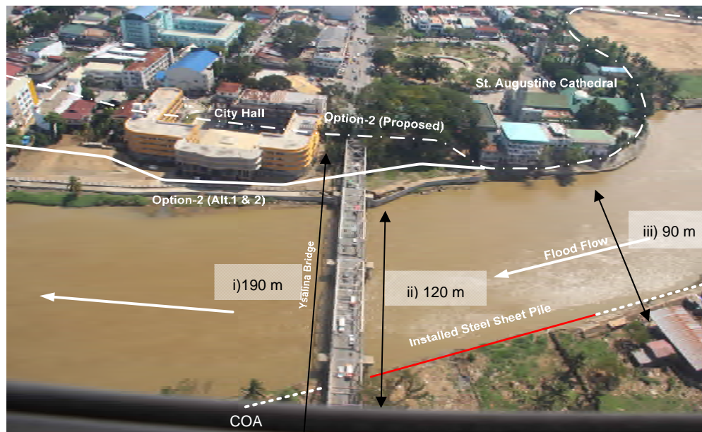
Note: i) Bridge length between abutment ii) River width of low water channel at present (between Piers No.1 and No.3) iii) The narrowest river section upstream of Ysalina Bridge
