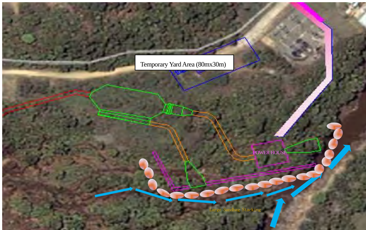
Figure 2-9 Outline of Temporary Facilities around the Powerhouse
