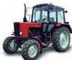
The wheeled tractor BELARUS 82.1 (4x4) is a universal agricultural tractor of drawbar category 1.4, powered by a 82 h.p. engine, intended for various farm jobs with mounted, semi-mounted and trailed machines and implements.
