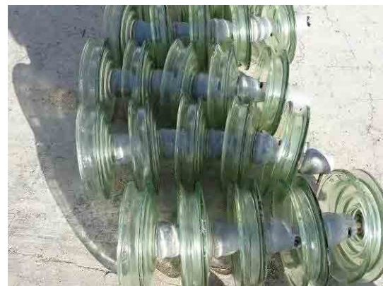
Figure 4-3 Glass Insulators (left: Russian-made, right: Chinese-made)
