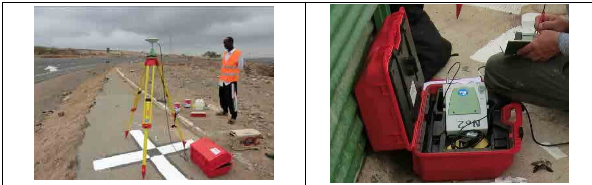
Figure 13 GNSS Observation (Left: GNSS observation; Right: Leica GS10 GNSS receiver)
