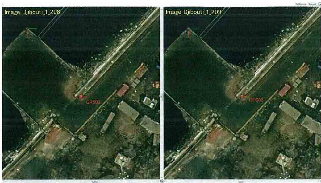
Figure 24 Automatic Observation of Pass Points and Tie Points
