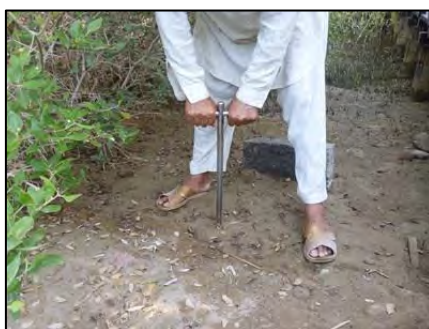
Figure 2.4.3 Collection of soil sample with core sampler
