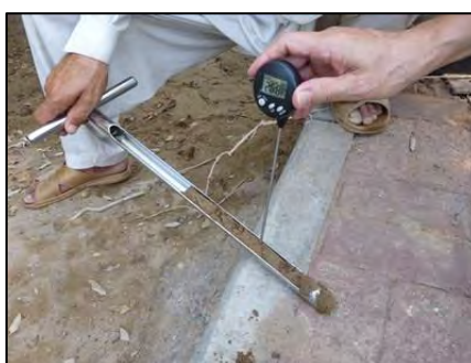
Figure 2.4.5 Measurement of soil temperature with soil thermometer
