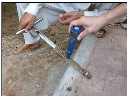
Figure 2.4.6 Measurement of ORP with ORP meter
