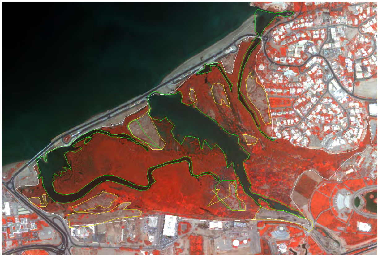
Fig. 5. GeoEye band 4, 2, and 1 color composite image of Qurm mangrove and surrounding areas recorded on September 18, 2012 with overlays showing the general area of the mangrove forest (white) wadi and water (green) and open flat or bare soil (brown).
