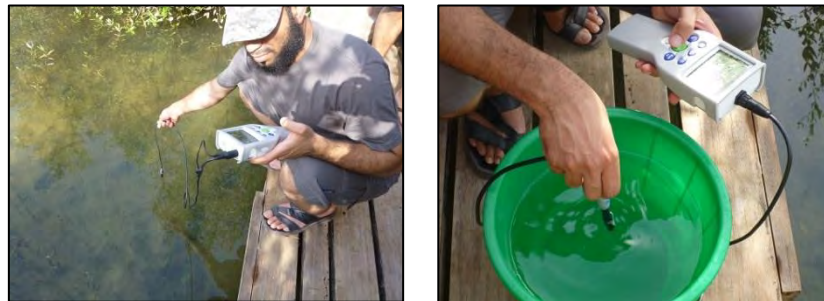
Figure 2.4.2 Measurement of water quality with portable water quality meters
