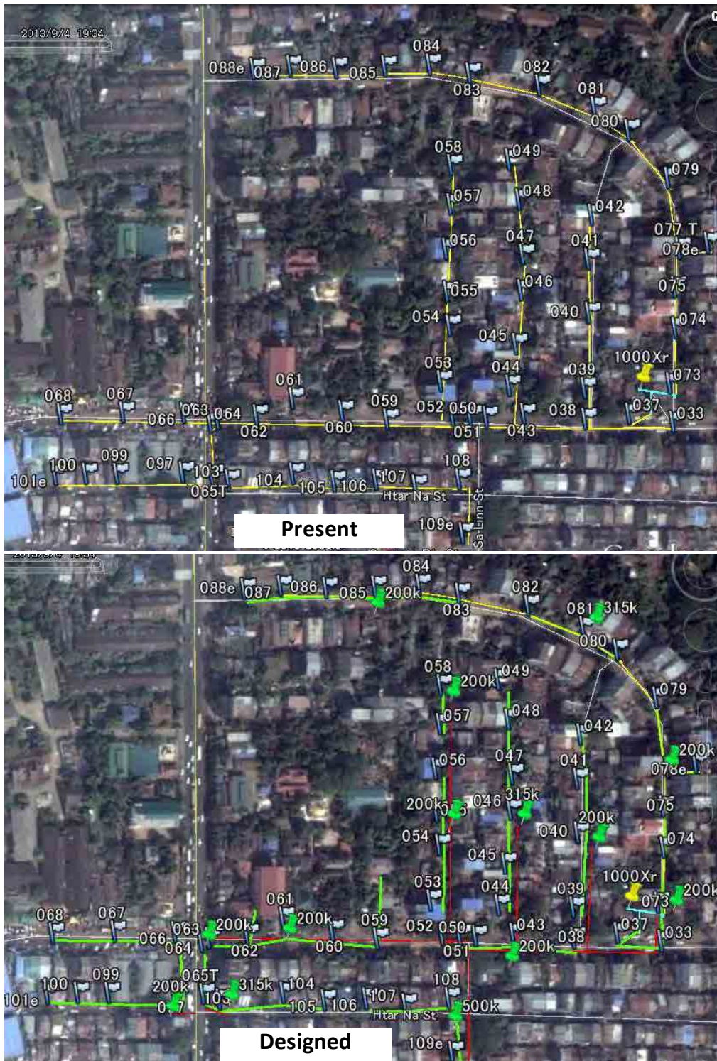
Figure 5-4: Drawings before and after the design of multi-transformer system in an overcrowded residential area.
