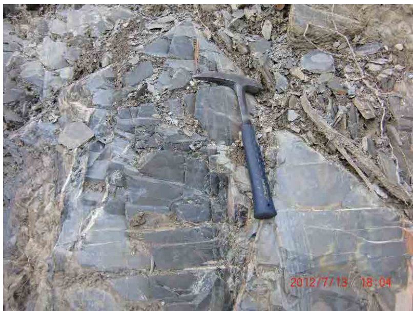
Figure 1.10: Light grey, laminated and fractured shales at the dam site, at waypoint WPT081.
