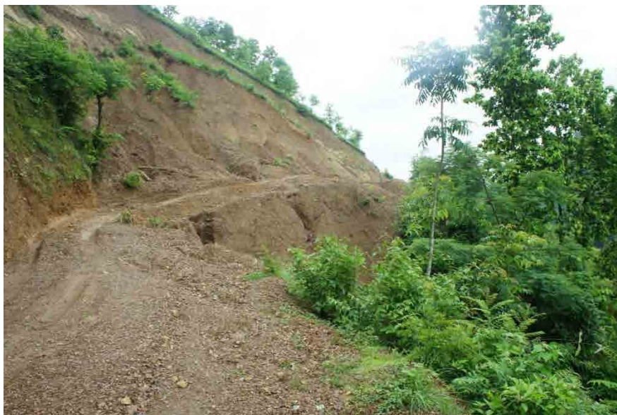
Figure 1.14 Photograph showing a large landslide on highly weathered slate (almost converted to residual soil) near location 034 (Figure 7.2).
