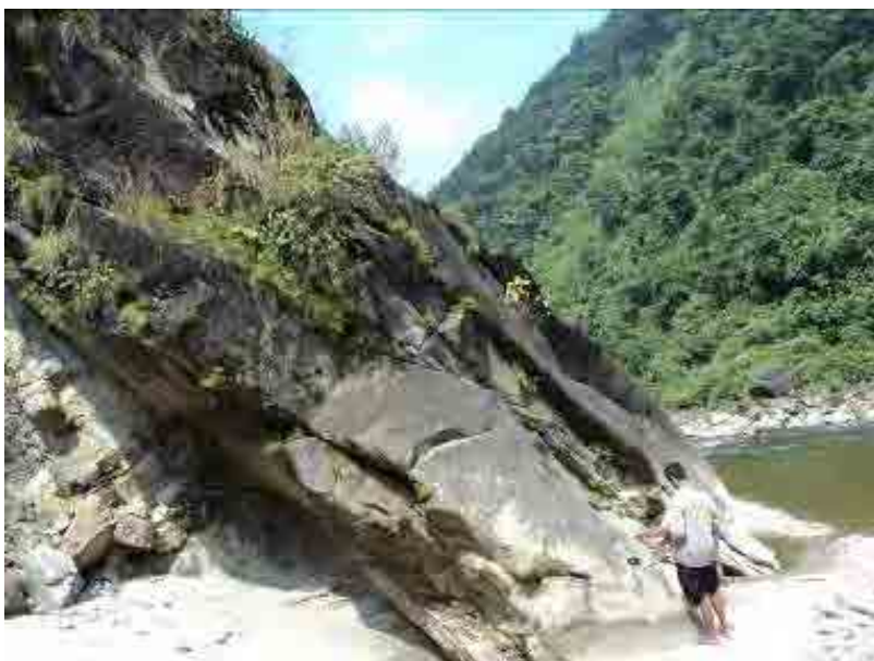
Photo 1.3: Jointed sandstone on the left bank of Kokhajor Khola in intake area
