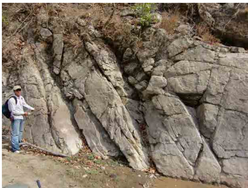
Figure 1.10: Thickly bedded and jointed sandstone beds, at left bank of dam site, at waypoint NAU03. View to SE.
