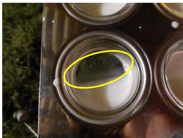
Picture2-8 Test Result from Milk Sample from Bucket (Clump Positive)
