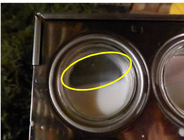
Picture2-7 Test Result from Milk Sample from Caw (Clump Negative)
