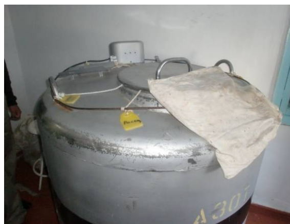
Picture 6-10 Depositing tank for frozen semen
