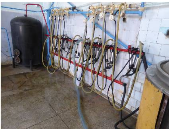
Picture2-12 Pipeline Milker
