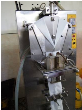
Picture2-32 Plastic Bag Packing Machine
