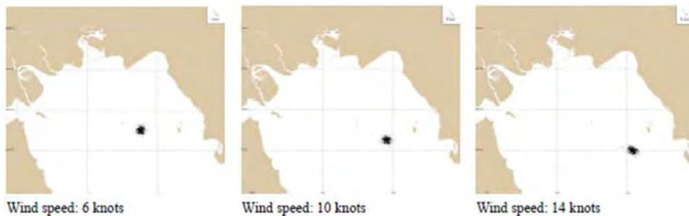
**Figure 1.3-4(1) Trajectory of the spilled oil after 5 days at Aboozar oil field (Season: Feb-Oct, Wind direction: Northwest)**
