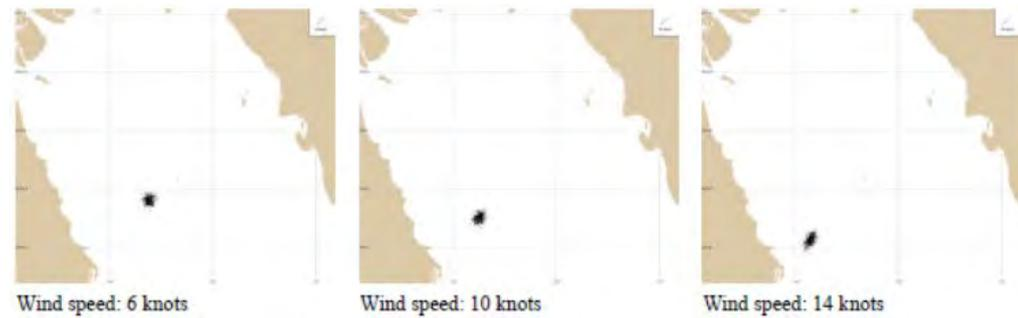
**Figure 1.3-5(2) Trajectory of the spilled oil after 5 days at Foroozan oil field (Season: Nov-Jan, Wind direction: Northeast)**
