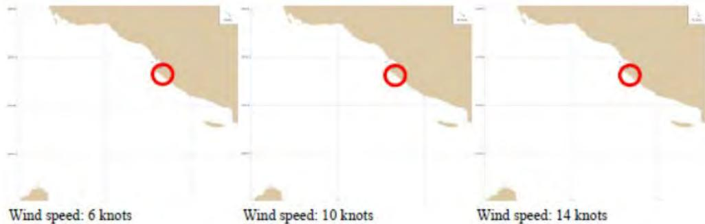
**Figure 1.3-8(1) Trajectory of the spilled oil after 5 days at the SPM system at offshore for loading of condensate, Assaluyeh (Season: Feb-Oct, Wind direction: Northwest)**
