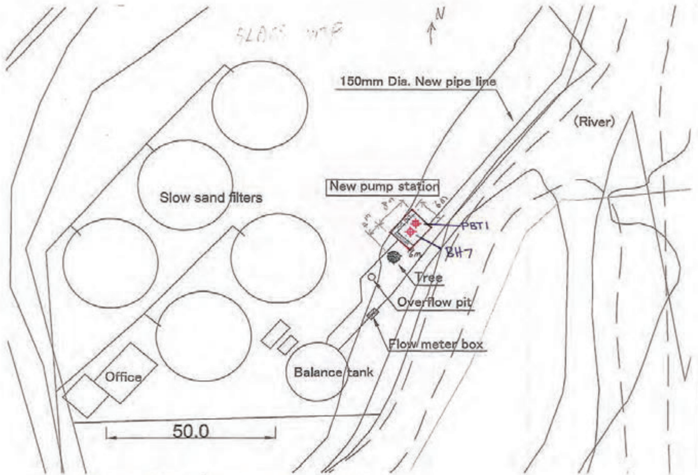
Figure 4: Existing Alaoa water treatment plant
