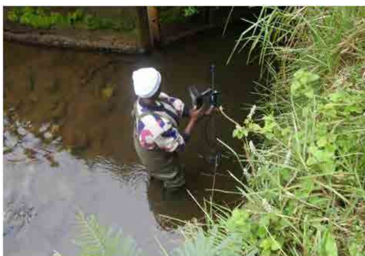
Figure 16: Discharge measurement by ADV
