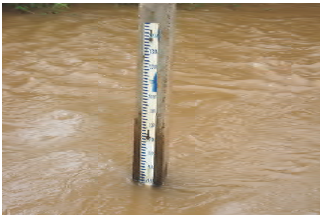
Figure 9: Staff gauged installed on concrete post
