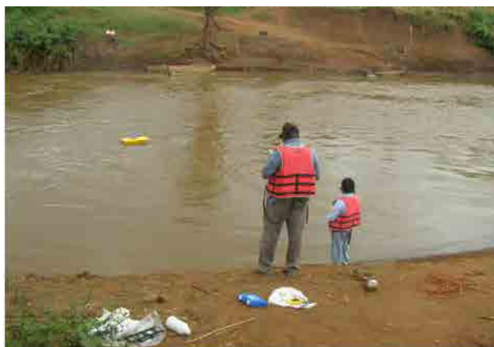
Figure 15: Discharge measurement by ADCP
