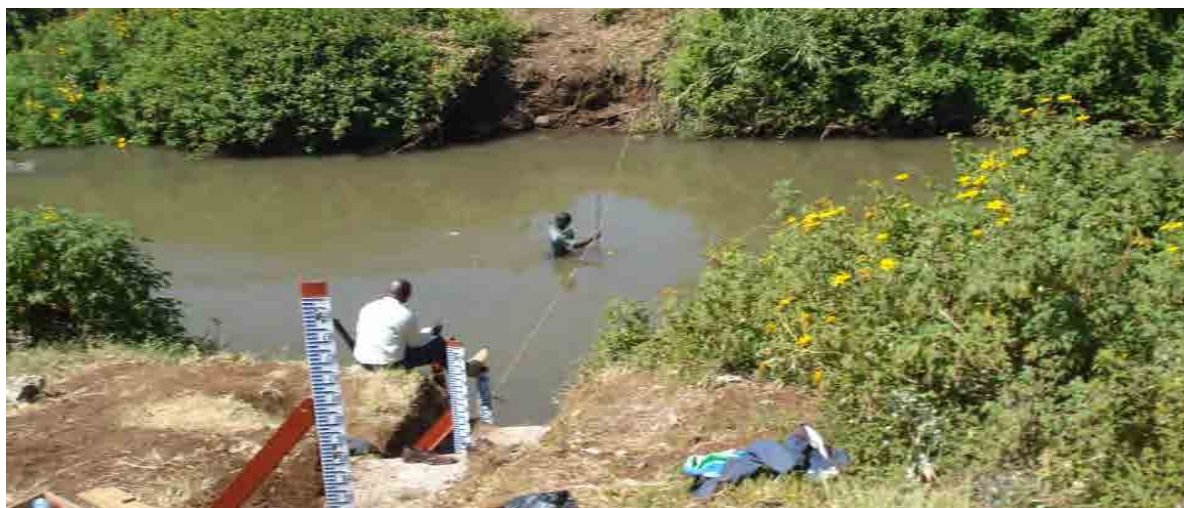
Figure 13: Current meter gauging by wading
