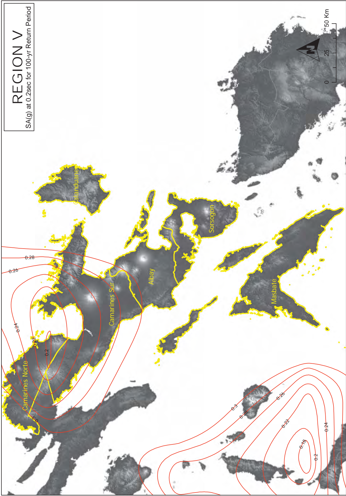
Figure 2A-149 Region V map of spectral acceleration at 0.2 sec. for 100-year return period
