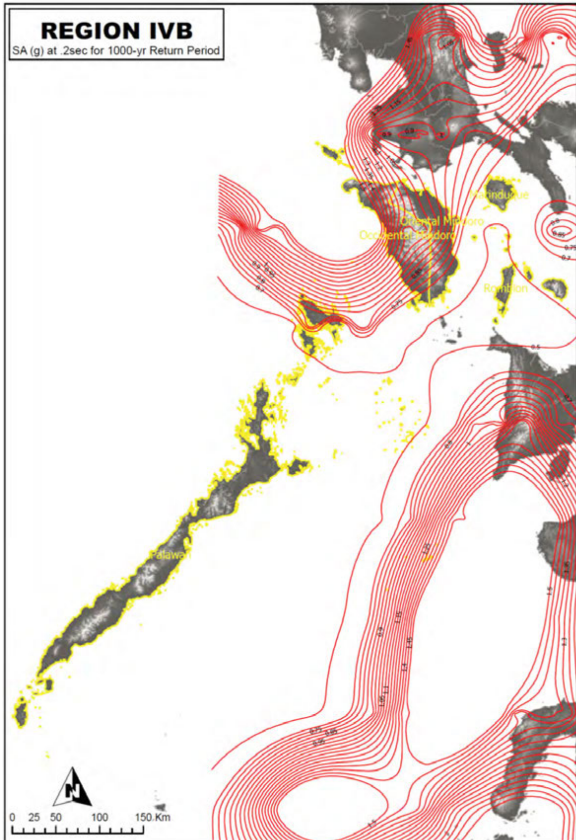
Figure 3B-27 Horizontal Response Spectral Acceleration Coefficient at Period of 0.20-sec ( S_S ) for Level 1 Earthquake Ground Motion (Region IV-B)
