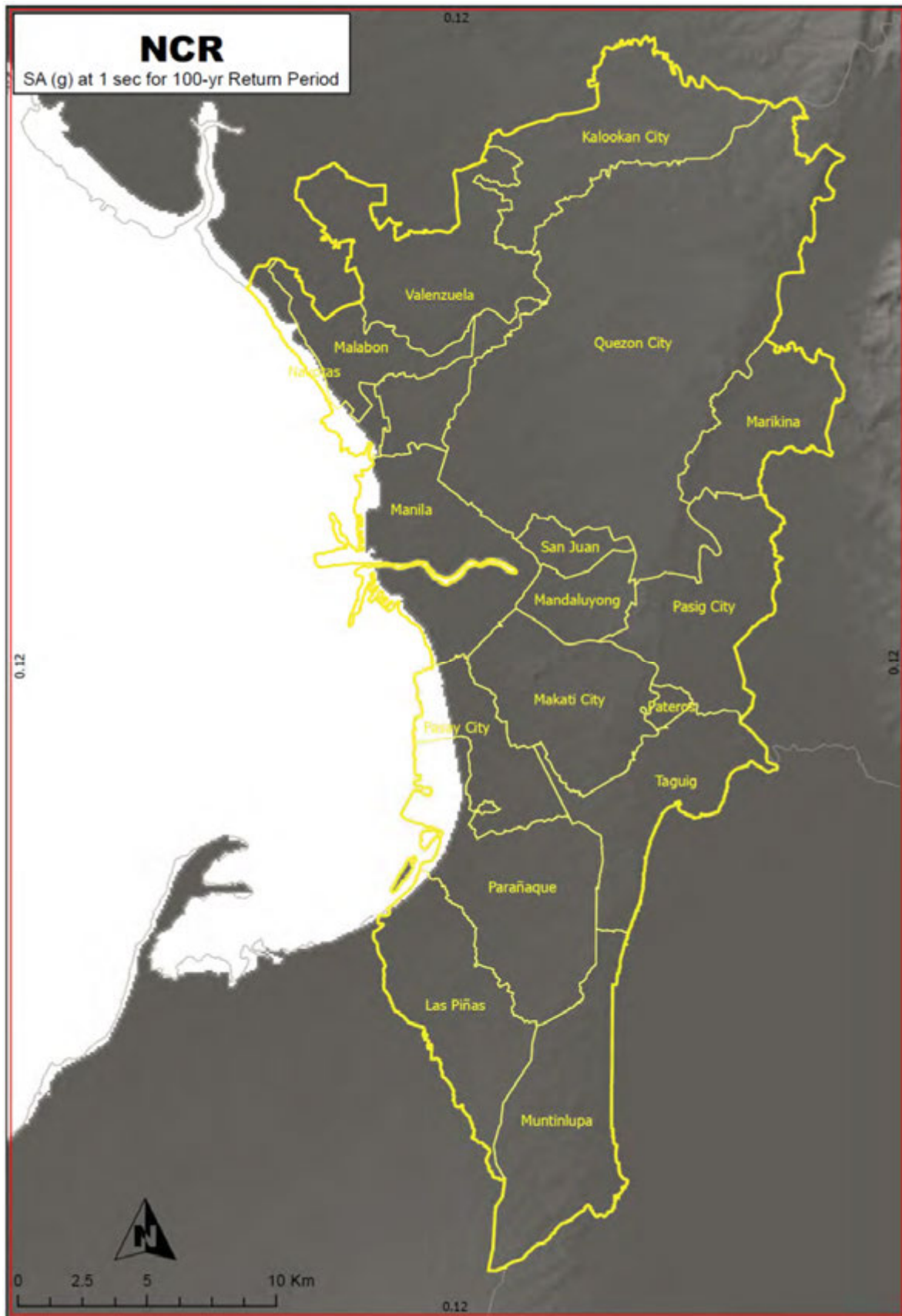
Figure 3A-42 Horizontal Response Spectral Acceleration Coefficient at Period of 1.0-sec ( S_T ) for Level 1 Earthquake Ground Motion (NCR)
