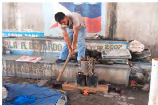
Generation of Seismic Wave by Hammer
