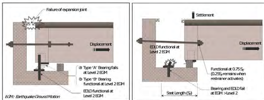
(b) Performance under design earthquake (Level 2 EGM)
