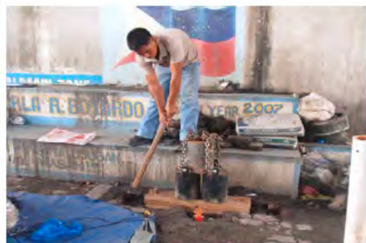
Generation of Seismic Wave by Hammer
