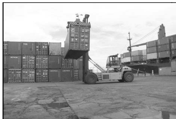
Photo 2.2.2.2-2 Container Handling Operation in the Yard by Top Lifter
