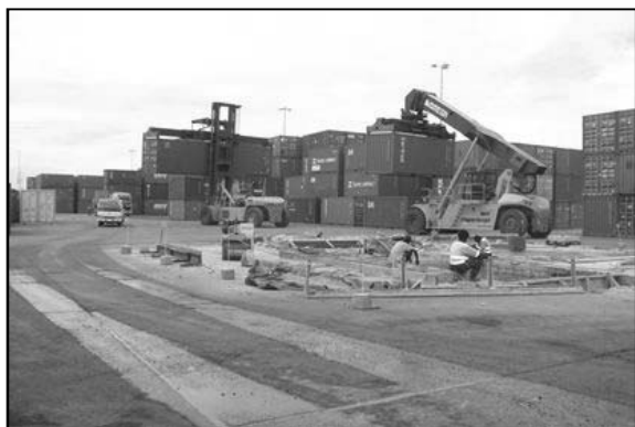
Photo 2.2.2.2-1 Container Carrying Operation between Berth and Yards by Top Lifter and Reach Stacker
