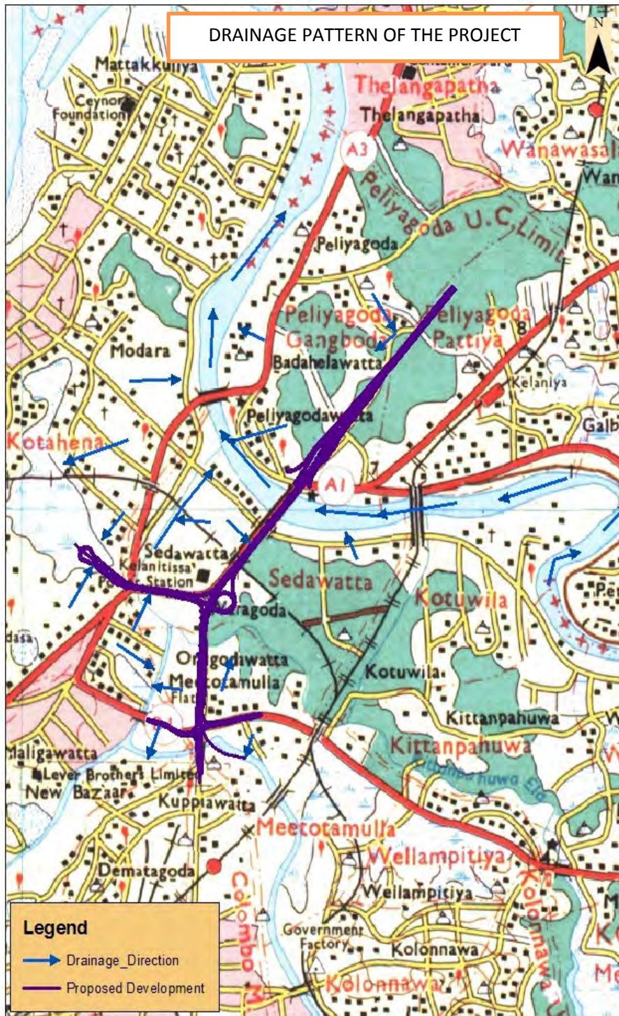
Figure 4-8 Drainage Pattern of the Project Area
