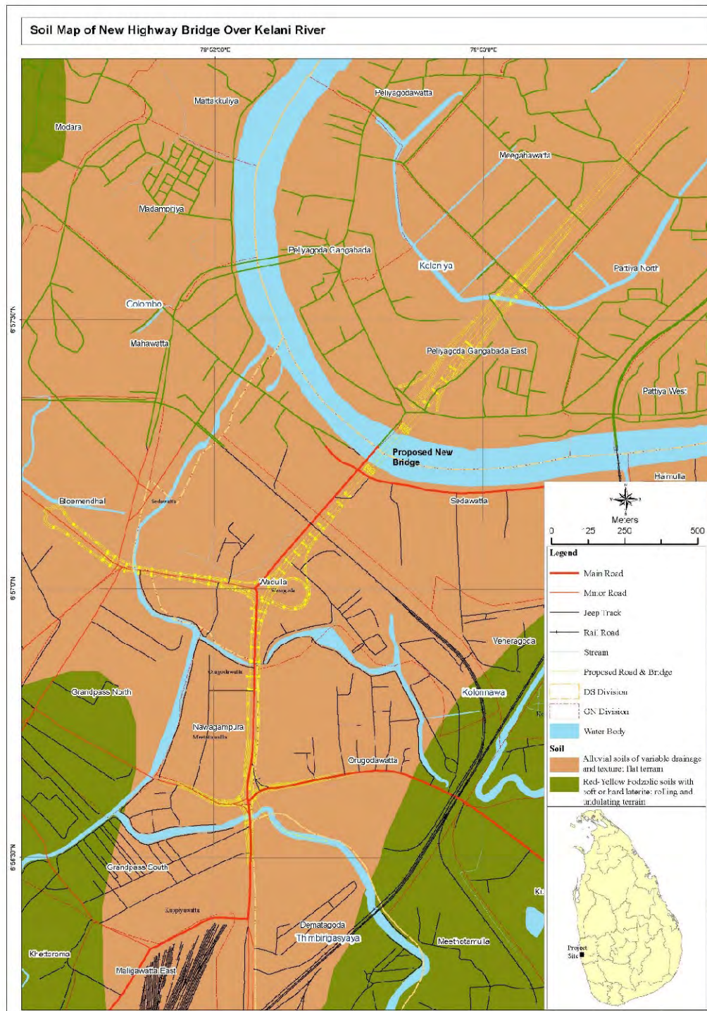
Figure 4-2 Soil Map of the Project Area (Source: Panabokke C- Soils of Sri Lanka)
