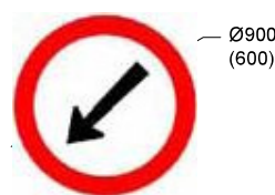
2. 3. 6 PASS THIS SIDE LEFT SIDE
