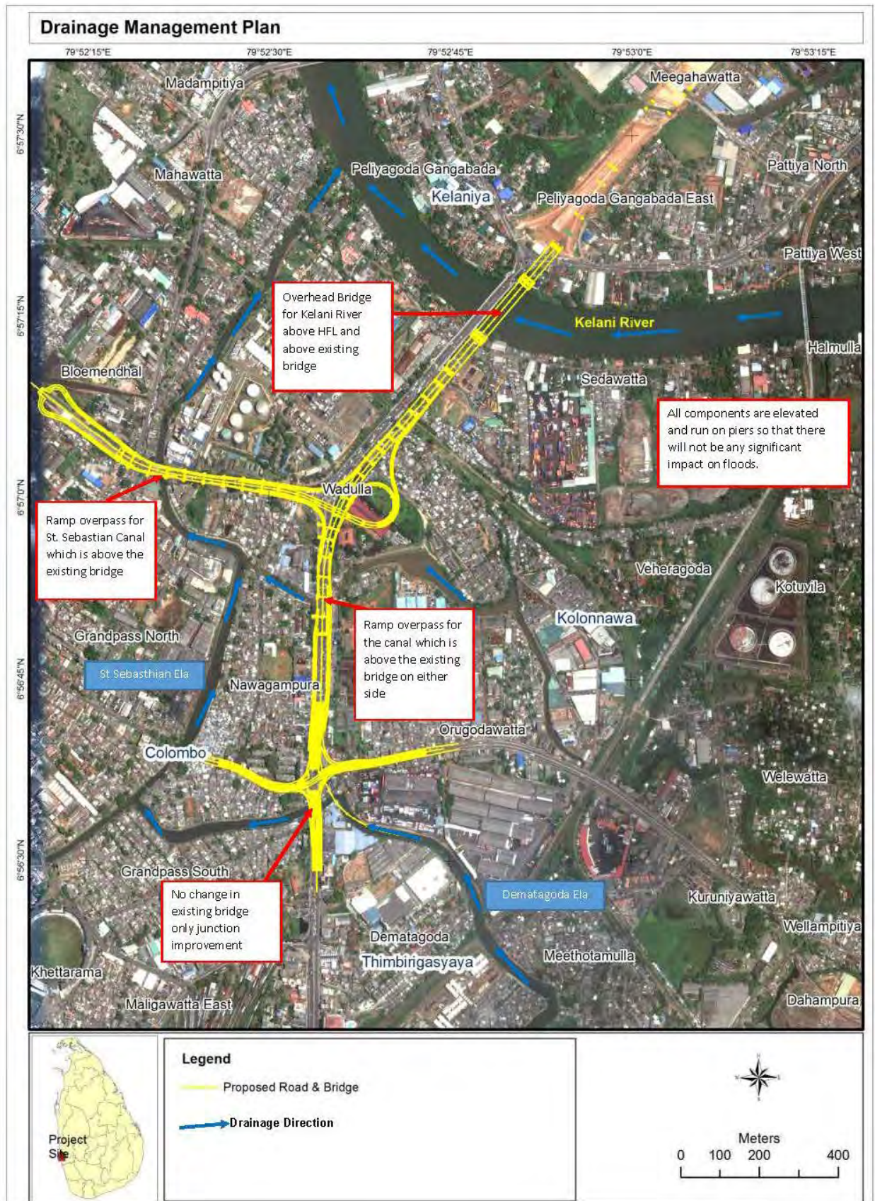
Figure 6-9 Drainage Management Plan
