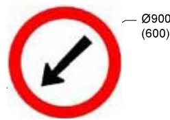
2. 3. 6 PASS THIS SIDE LEFT SIDE
