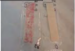
Result of E. coli test for typical domestic water at a colony in Dhaka
