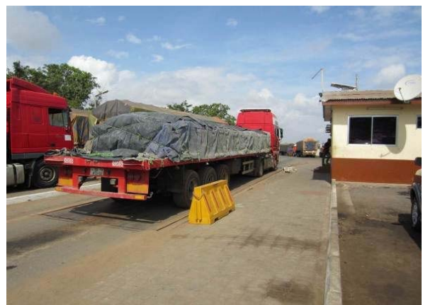
Not each axle but total weight is measured at weighbridge.
