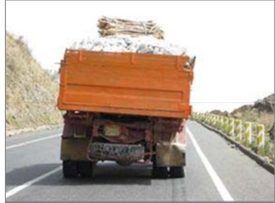
Photograph 4-7. The speed is less than 5km/h. This is because it is fully loaded with crushed stone and vertical gradient is around 10% .Asphalt begins to flow on a passage line of the right tire.
