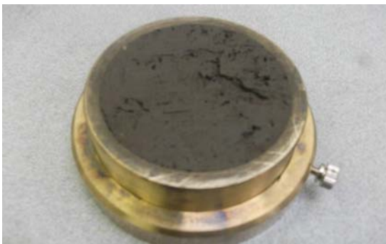
Photograph 4-17. A test specimen of 20mm of the black cotton soil expands to 35mm 96 hours later (Condition is before immersion in water)
