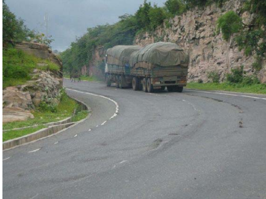
Photograph 4-6. The speed is less than 10km/h because it is the small section of a vertical gradient is around 7%, and small curve radius.
