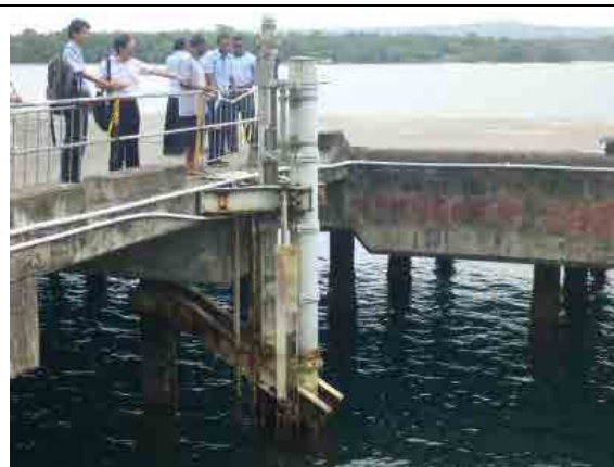
Existing tidal gauge owned by BOM (Efate Island)
