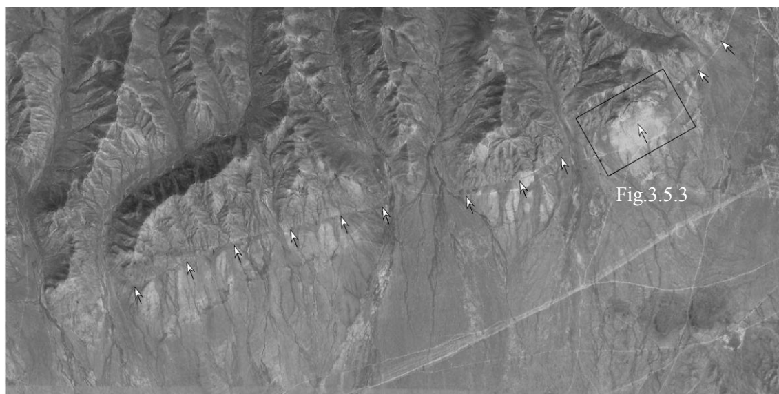
Figure 3.5.2 The Hustai fault seen on satellite images. Arrows indicate fault trace. (Satellite images are from Google Earth)
